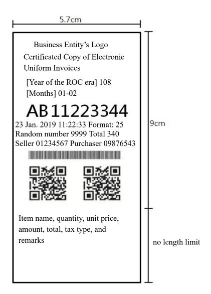
Figure 1-3. Certificated Copy of Electronic Uniform Invoices with "REPRINT" note (example)
